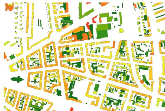
Figure: Spatial distribution of total energy demand of electricity. Values in kWh/(m²<sub>A,B</sub>\*a)
