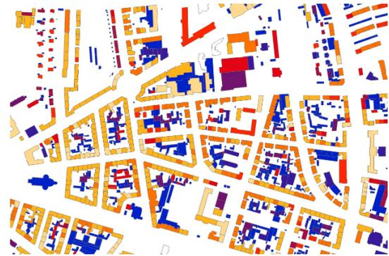
Figure: Spatial distribution of total energy demand of thermal energy. Values in kWh/(m²<sub>A,B</sub>\*a)
