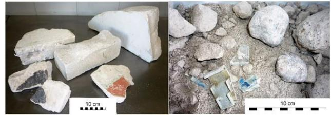
Figure 8: Aerated concrete waste to be recycled
