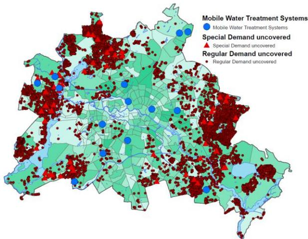
Figure 5: Selected locations of mobile treatment plants (blue dots) in case of a failure scenario of the Berlin water supply (Stallkamp et al., 2020)
