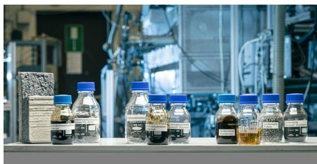
**Figure 3: Pyrolysis condensate from different plastic waste fractions**
