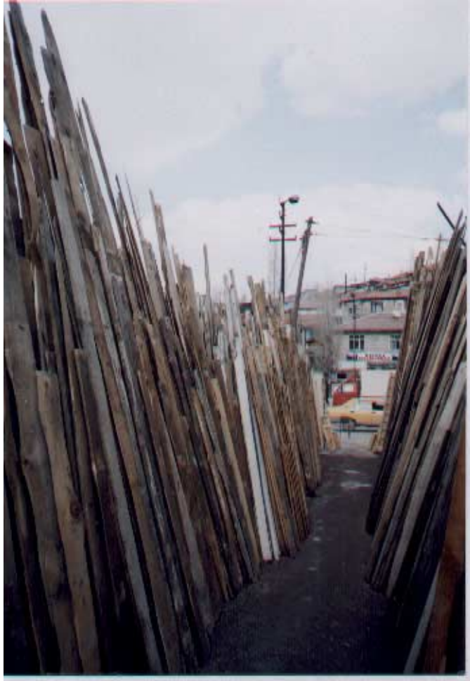
Figure 7. Timber recovered from the roofs of demolished buildings.
