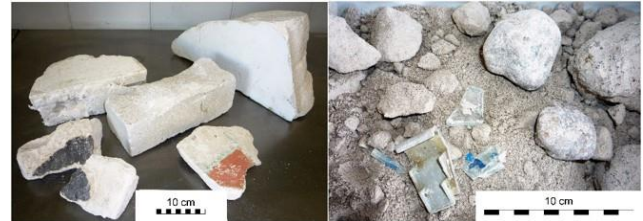
Figure: Aerated concrete waste to be recycled
