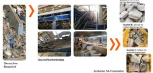
Figure 9: Provision of old aerated concrete in various grades of purity
