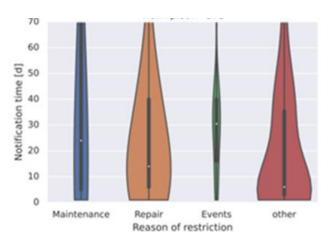
Figure 7: Distribution of warning time regarding the reason for closure of waterways based on Notification to Skippers at the West German Canal Network (n = 573)
