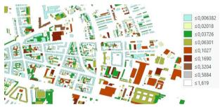
Figure: Distribution of steel in the Oststadt Karlsruhe. Values are in  $Mg/m^2_{A_B}$
