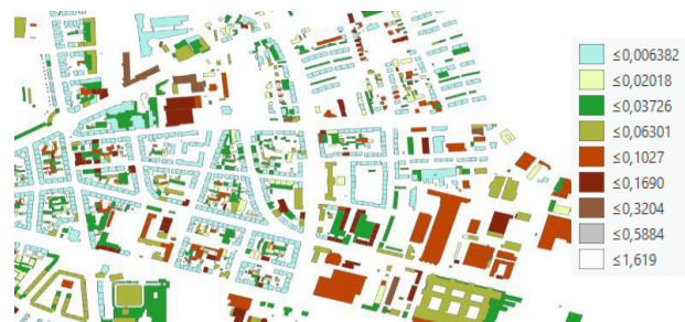
Figure: Distribution of steel in the Oststadt Karlsruhe. Values are in Mg/m 2 A B
