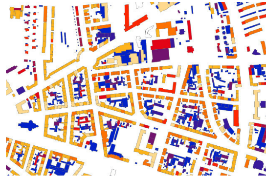
Figure: Spatial distribution of total energy demand of thermal energy. Values in kWh/(m 2 A B *a)
