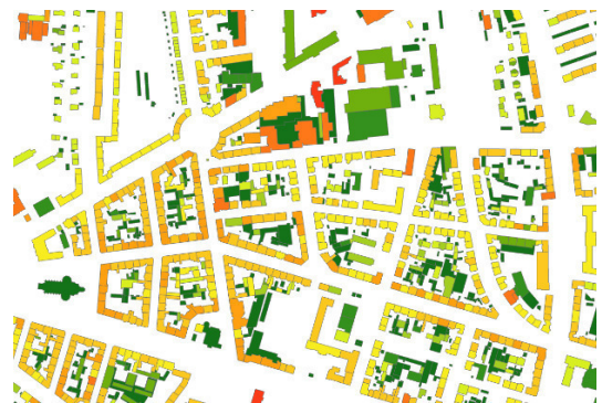
Figure: Spatial distribution of total energy demand of electricity. Values in kWh/(m 2 A B *a)
