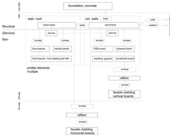
Figure 10: Vandkunsten 2007, Kvistgård, assembly diagram. Structural members and the complete skin layer are integrated in prefab panel elements except for the on-site façade cladding covering the connections.
