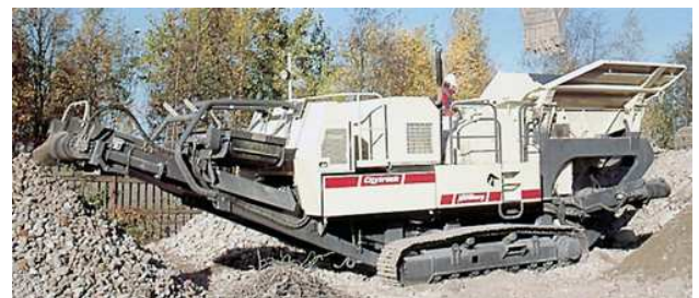
Figure 2: Mobile construction waste treatment plant made of a primary screen, an impact crusher and a magnet (< www.aufbaukoernungen.de/ziele.html > 08/12).
