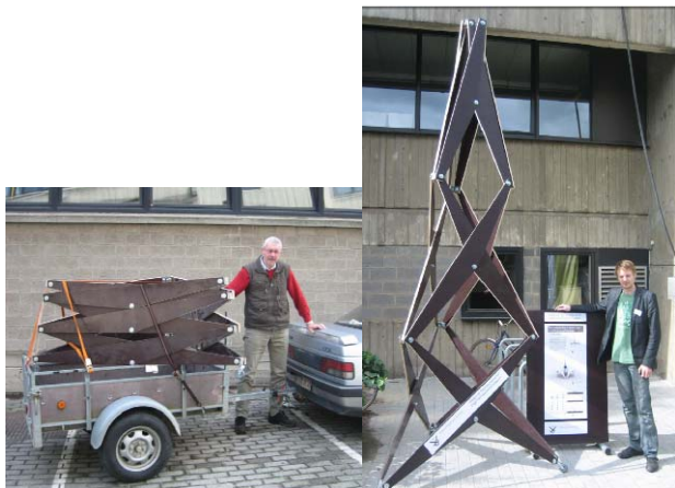
Figure 20: Compacted and deployed state of the proof-of-concept scale model
