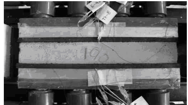
Figure 19: Sample holder of the thermal mass measuring device (sample between two thermo-regulated plates).
