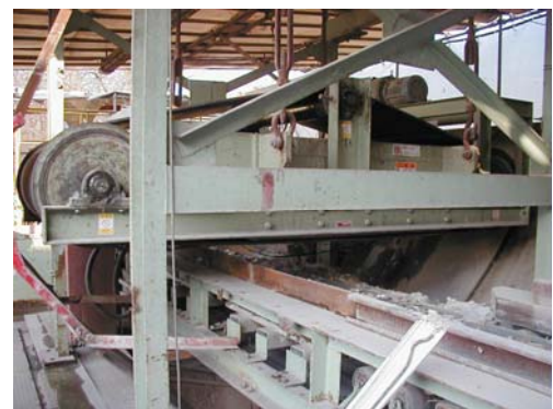
Photo 6 Metal removal by magnetic separator
